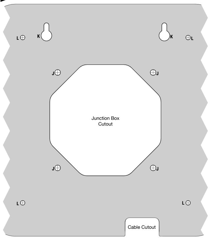
Use this template for drilling. Refer to instructions on reverse for hardware and installation.
