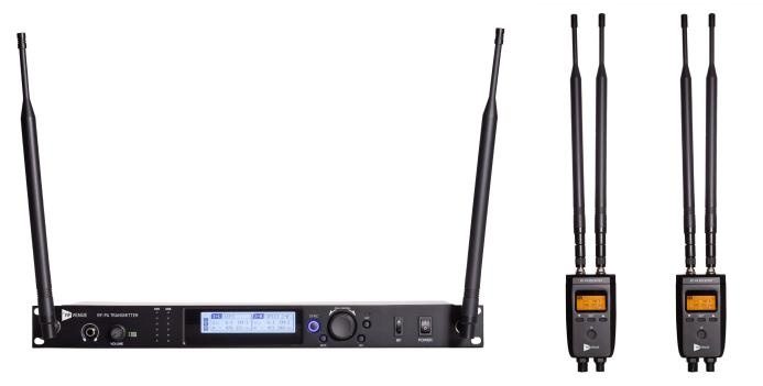
The RF Venue RF PA Extension Kit is your professional-grade solution for wirelessly extending PA audio. Using tried-and-true analog FM stereo transmission in the 470-506 MHz UHF band, it delivers robust, clear sound to those hard-to-reach locations. Onboard per-receiver delay (up to 800ms) ensures perfect audio synchronization across all your satellite speakers.
