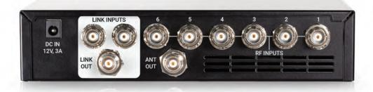
The COMBINE6 HDR, is a compact, half-rack unit that streamlines your IEM setup. It combines up to 6 IEM signals into one, eliminating the "antenna farm" problem. Imagine a single, powerful antenna transmitting a crystal-clear mix to all your performers.
