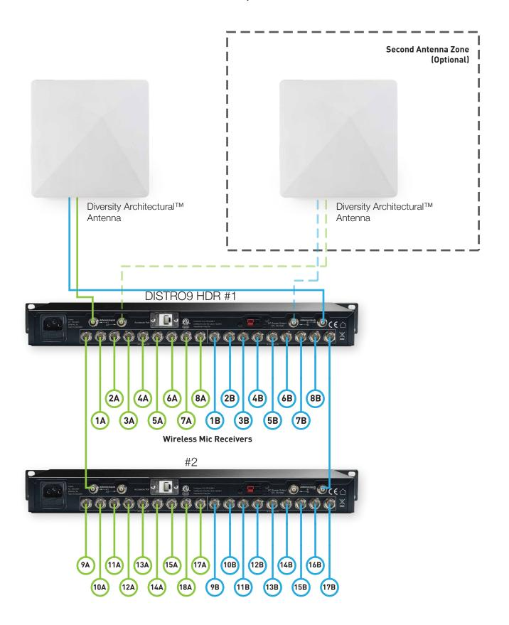
\*DISTRO9HDR #1 (Master) can feed signals to up to 9 additional DISTRO9HDRs. Each connected DISTRO9HDR can feed up to 9 receivers. \*Note: All outputs are equivalent. Any "A" can be paired with any "B" and any pair can be cascaded.
