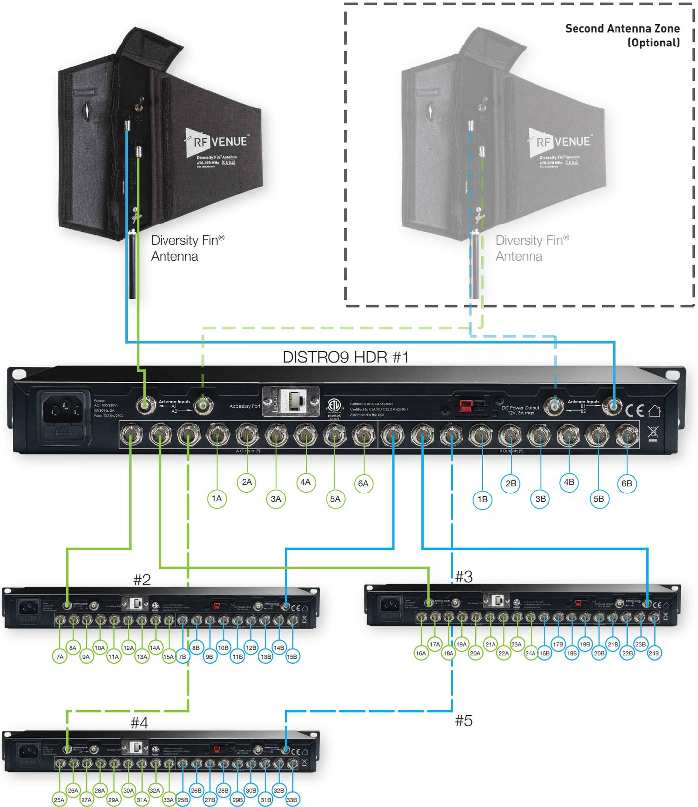
\*DISTRO9HDR #1 (Master) can feed signals to up to 9 additional DISTRO9HDRs. Each connected DISTRO9HDR can feed up to 9 receivers.
