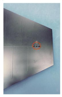
If you have a DFIN that is painted, scrape away the paint from the solder where the connector will be replaced.
